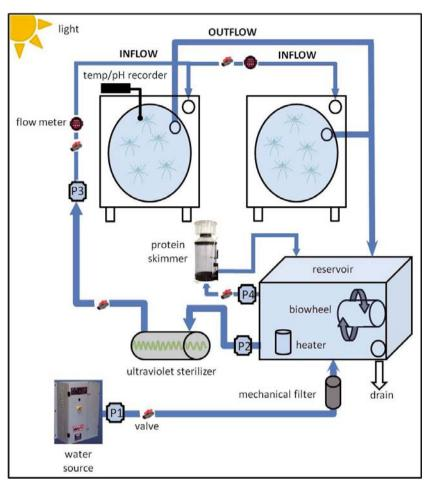
**Fig. 2.** Flow diagram for the design and operation of plankton kreisel tanks and their associated supporting components (e.g., pumps, P1, P2...) in a semi-closed seawater system. Water turnover for this system was calculated at ~75% of total volume per day and was sourced from instantaneous temperature-controlled seawater (25.0 °C) at a salinity of 30–35 psu. See text for component details.
